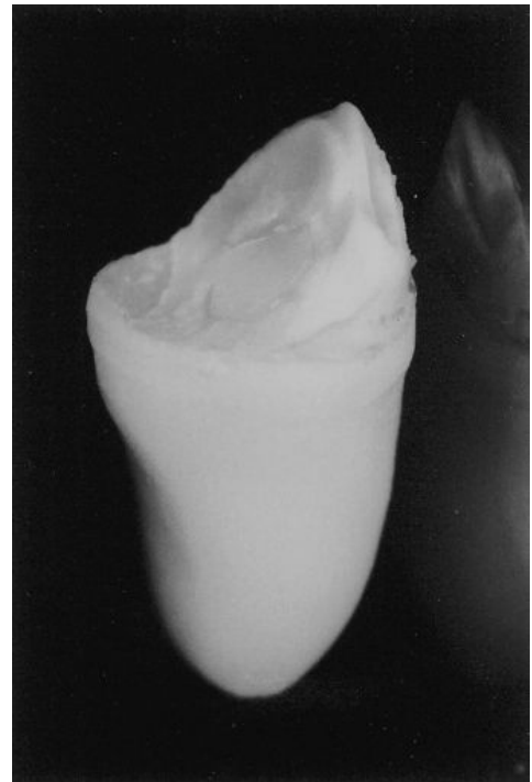
FIG 5. Fracturing of the root and RCIPC post in the artificial oral environment (group C).
