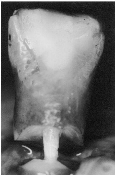
FIG 7. Failure of a specimen in the Zwick testing machine (group D).
