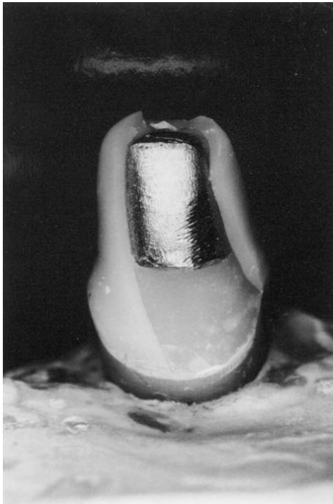
FIG 3. Fracturing of a PROCERA coping in the artificial oral environment (group A).
