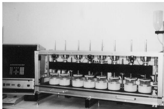
FIG 1. Artificial oral environment (Willytech).
